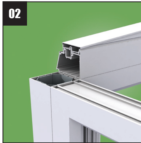
02 Each firing is 45mm longer than the internal frame projection. When cutting the firing, always do this at the back (rear) and ensure that all elements are in aligned.
