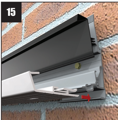
15 Attach undercladding, having first sub assembled the ventilation button (separate installation leaflet provided in vent button kit)
