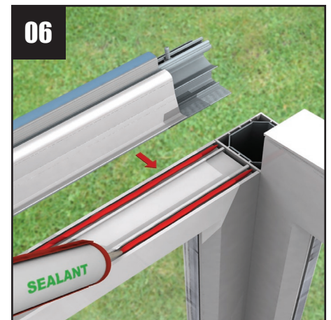
06 Take the eaves beam and make sure the head of the front frame is siliconed.
